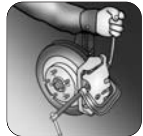
6 Open bleeder and then compress piston. Do not hammer to set pads into place.
